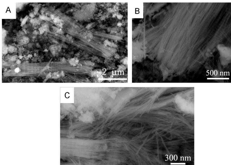
Fig. 1. SEM images of BNBs: (A) Typical SEM image of large-area BNBs, (B) The side view of BNBs and (C) Magnified image of the BNBs.
