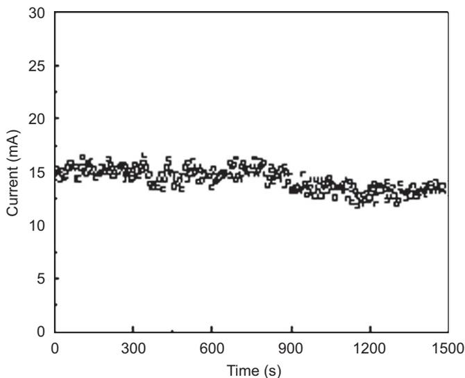
Fig. 5. Typical emission stability curve of BNBs film at high current density.
