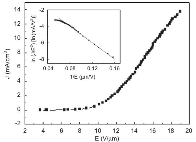
**Fig. 4.**  $J$ - $E$  curve from large-area BNBs film. The inset is the FN plots of the sample.
