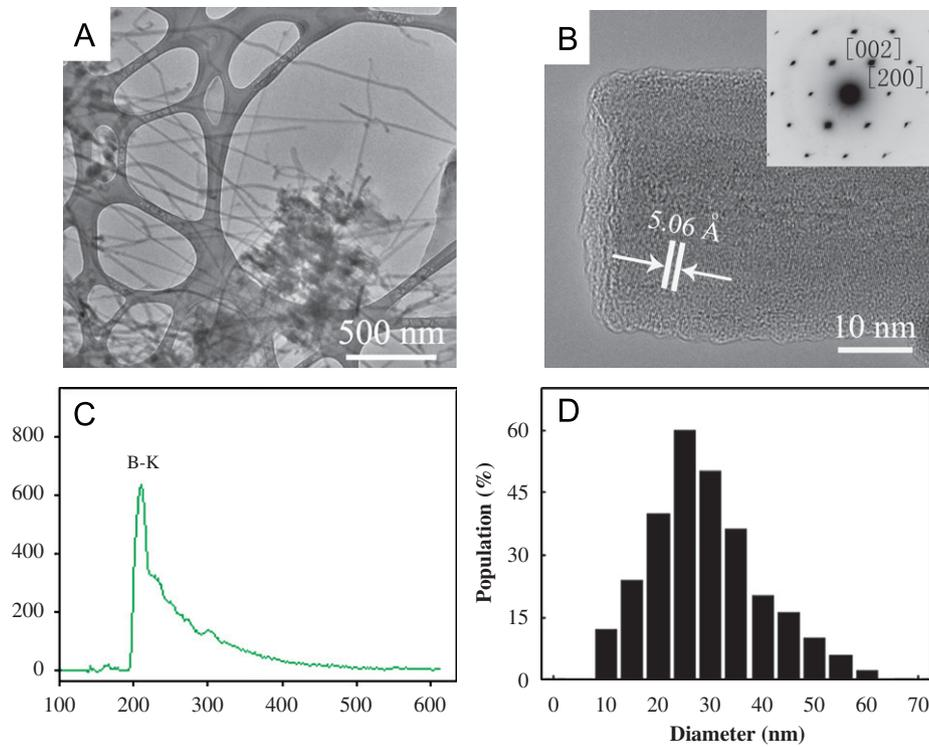
**Fig. 2.** TEM and HRTEM images taken from BNBs. (A) Typical TEM image of BNBs. (B) HRTEM image of a boron nanowire in the bundle. The inset is the corresponding SAED pattern. (C) The EELS spectrum of a typical boron nanowire. (D) The diameter distribution histogram of the boron nanowire in the bundles.
